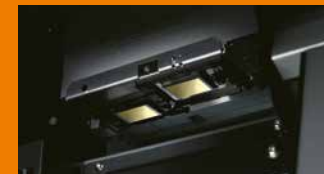
Dual print heads in staggered formation.
